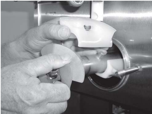
Figure 22. Auger Shaft Removal
