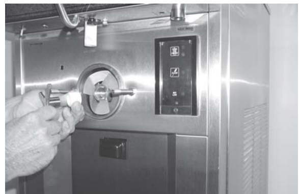
Figure 21. Removing Auger Support
